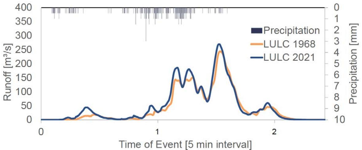
**Figure 11.** Modelled runoff of the hydrological model HEC-HMS. The two days rainfall event from February 2019 (5-minute resolution of rainfall series) was modelled with the LULC 1968 (yellow) and the LULC 2021 (blue).
