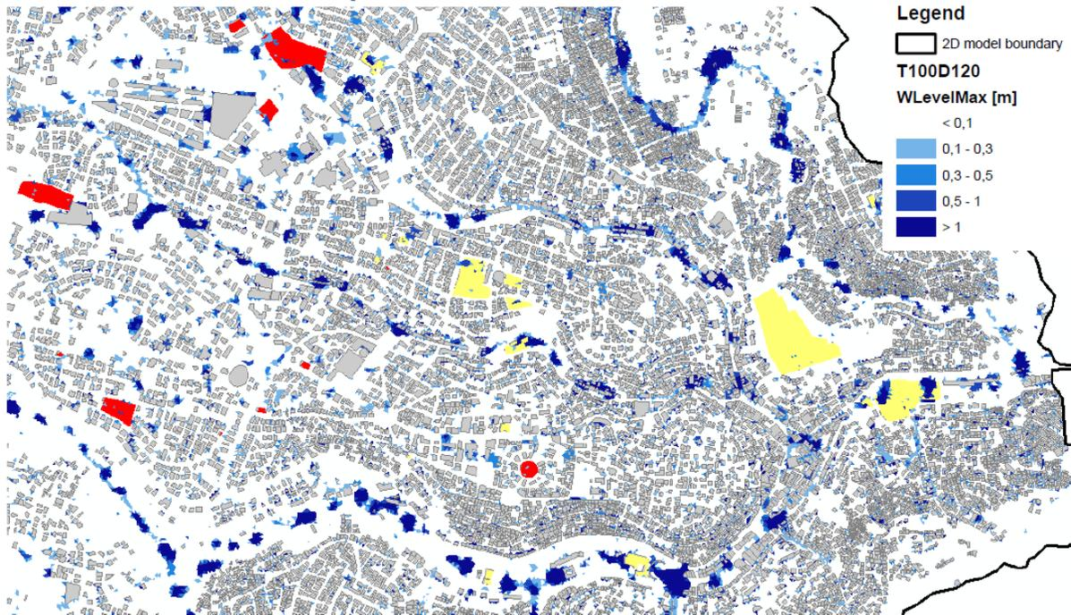
**Figure 10.** First risk map for Downtown Amman. Results of the hydro-dynamical 2D simulation with the model HE2D/FOG2D and building usages with a high (yellow) and a very high (red) damage potential are shown.
