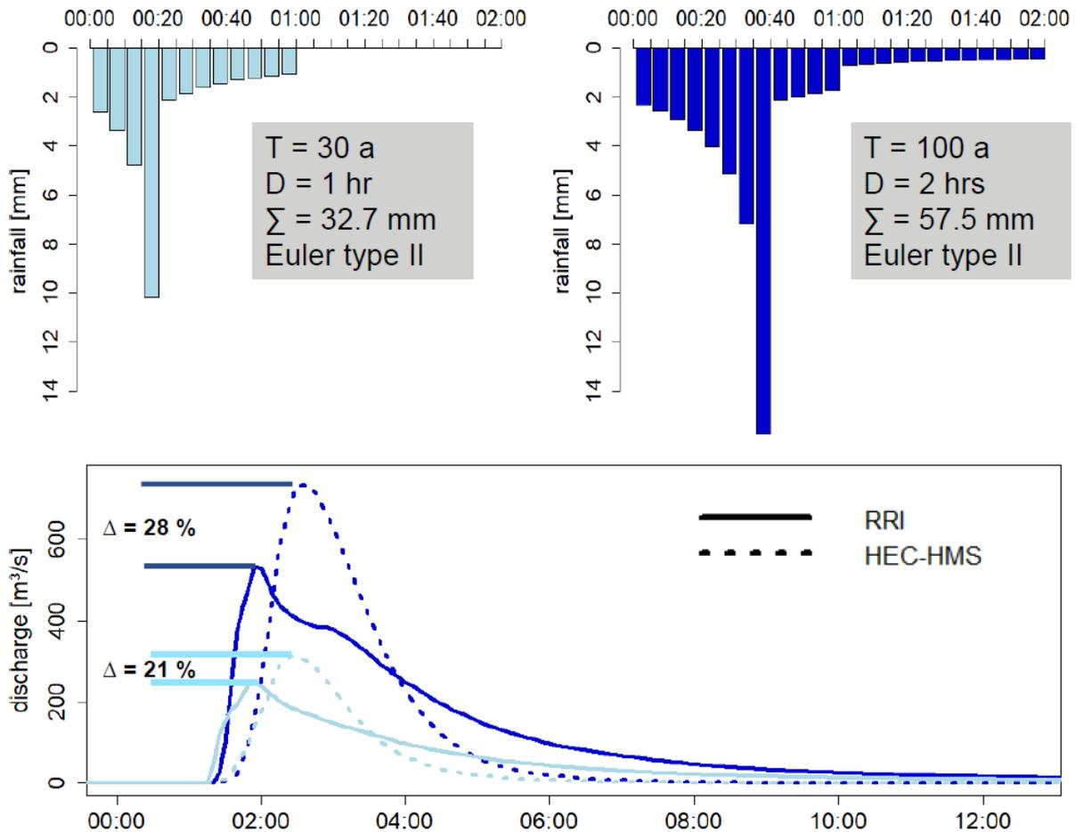
**Figure 13.** Runoff curves modelled with HEC-HMS (dotted) and RRI (solid) at the outlet of the Wadi Musa catchment ( $A_E = 130 \text{ km}^2$ ) for two design storm events with different return periods (T) and durations (D).
