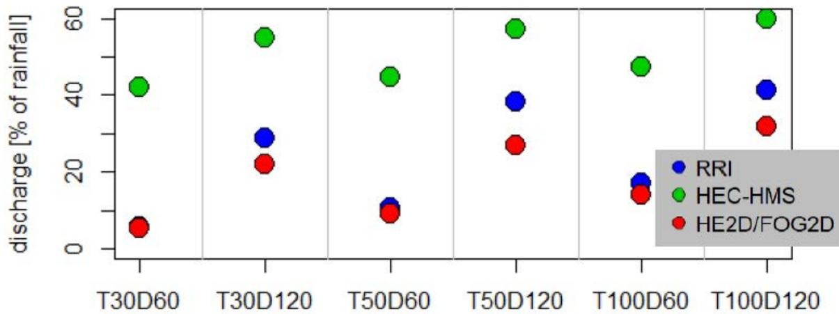
**Figure 12.** Total runoff volumes modelled with RRI, HEC-HMS and HE2D/FOG2D for design storm events with different return periods (T) and durations (D) for a subbasin of the Wadi Musa catchment ( $A_E = 18.5 \text{ km}^2$ ).
